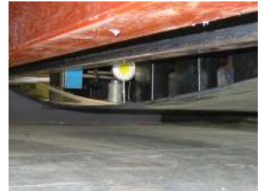
Testing the Glass Deviation
