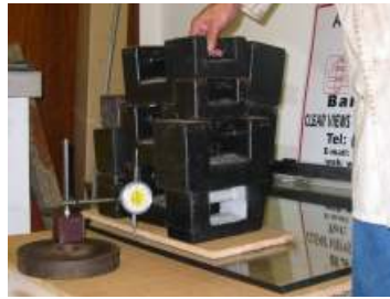
SABS Testing on Balustrade Glass
