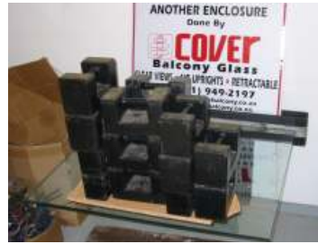
SABS Testing on Balustrade Glass
